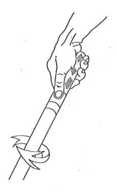
Close release valve by rotating handle fully clockwise until it reaches the built-in stop.
