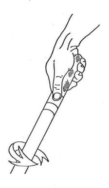
Open release valve by gradually rotating handle anti-clockwise until load begins to descend. The rate of descent can then be controlled as required.
