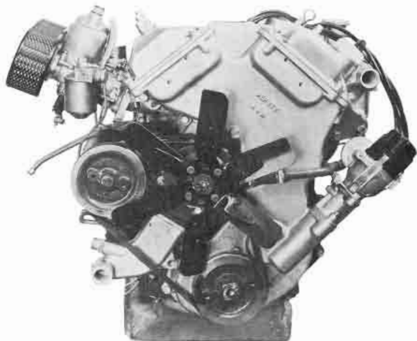
Front view of the early Twin-Cam production engine, showing that it was at least as wide as it was deep. The distributor drive was located in the new cast front cover ( BL )
