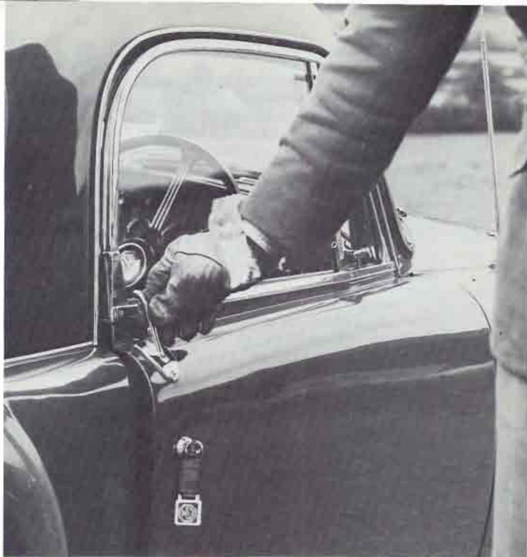
The very neat exterior handle detail of the MGA Coupe's doors. The same feature was, of course, used on Twin-Cam coupes. Tourers never had exterior handles of any type ( BL .)
