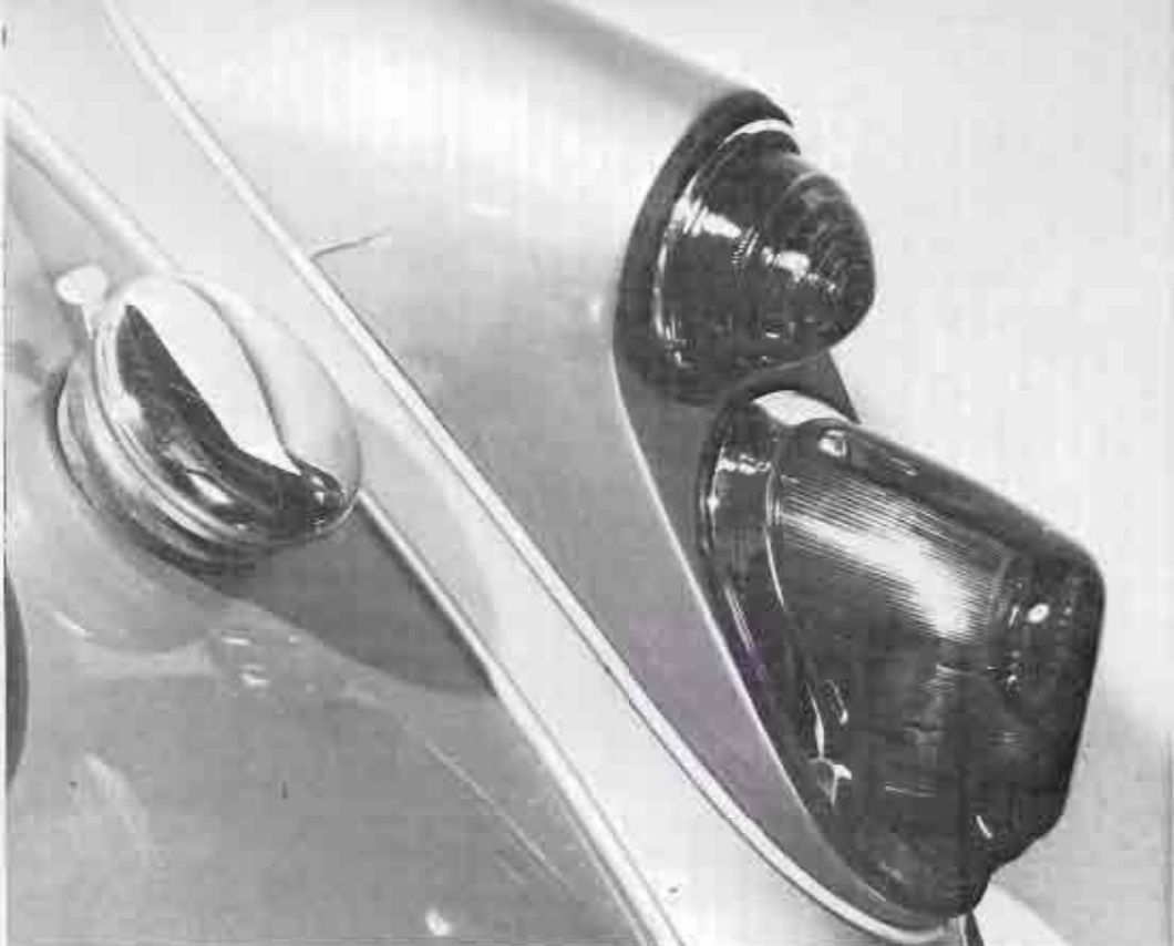
One identification point which pinpoints a late-model, 1959/60, Twin-Cam is the tail-lamp cluster, which was brought into line with the cluster specified for pushrod-engined MGA 1600s in the summer of 1959 ( BL )
